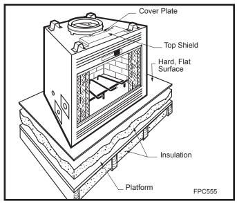
Fig. 8 Insulating between platform and fireplace.
